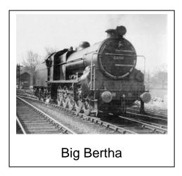
Modern steam engines were sufficiently powerful to haul trains up the incline without help from bankers. Early diesels sometimes required to be 'double headed' (hauled by two engines) to climb the incline but present day diesels do not require double heading or bankers.
